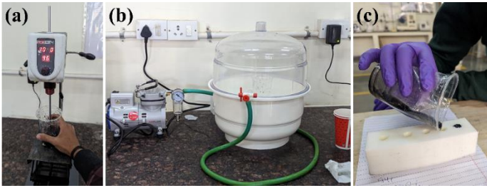
Fig. 3(a) Mixing of CCF with epoxy resin using an overhead stirrer, (b) degassing of epoxy resin, and (c) pouring of epoxy resin into silicone mold.
