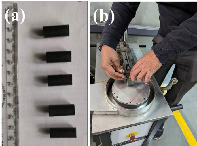
Fig. 4(a) The pin specimens made of cured EC, and (b) mounting of test pin into pin holder of tribometer.
